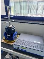
driven by a controller that follows a prescribed profile. Due to the complexity these systems, several issues may arise during the test. Digitalization offers powerful tools to predict the dynamic behaviour ahead of its physical execution. The so-called Virtual Shaker Testing (VST) environment can be built by coupling the controller with a time-domain dynamic model of the system under test (shaker + spacecraft) and it can be run to predict the results of the real test.
