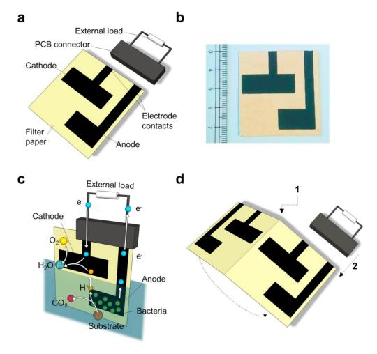
Chouler, Jon, et al. "A screen-printed paper microbial fuel cell biosensor for detection of toxic compounds in water."
