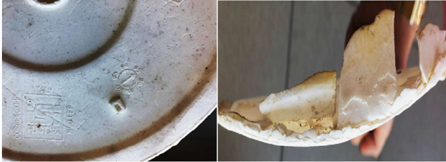
Fig. 13. Bottom part of fragmented plastic jar “PP95” (left). Residual lateral border with various fragments (right). Precursor of PP microplastics.
