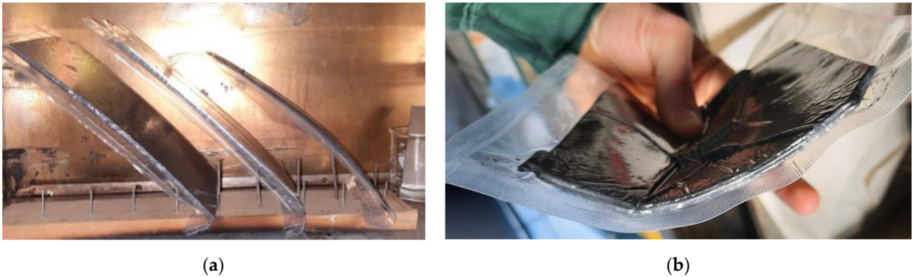
Figure 18. (a) Enveloped PA-SA/EG sheets from left to right 14, 12, 10 phr (effect of bending at 60 °C—angle 45°); (b) enveloped PA-SA/EG10 flexibility at 60 °C.
